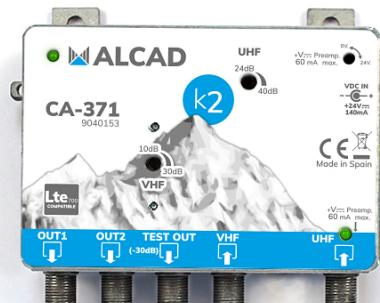
Head-end broadband amplifier with three inputs and two outputs. It has two UHF inputs with LTE700 rejection filters and another input for BI/FM/BIII/DAB. The two outputs have the same output level, with a maximum of 110 dB $\mu$ V, and facilitate the creation of star-shaped distributions using splitters.
